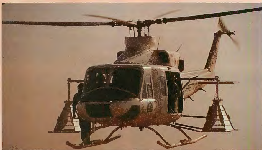
This United Nations helicopter was mounted with Ground Penetrating Radar to assist with inspection for proscribed weapons.
